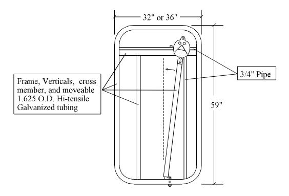
Closure is either manual or by cable pull from behind. Usually installed between two posts, or on the front of two posts. Can be clamped or welded. Closure size can be adjusted by sliding the moveable bracket on the bottom in or out. Designed to be used in maternity pens, usually in a corner along a fence, often with a swing gate on the other side to guide the animal going in or squeeze and contain the animal once locked.
